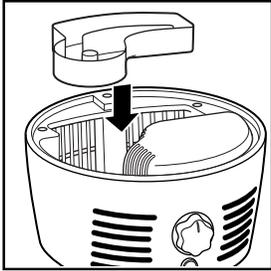
2. Place the filter on the water tray as shown.
