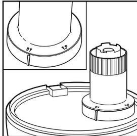
sure that the "LOCKED" arrows line up with the ridges on the fill neck.
