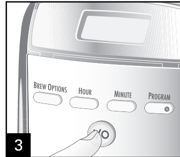
3 Press ON (I) . Turn OFF (O) after 30 seconds and wait 30 minutes. Press ON (I) . Turn OFF (O) when finished. When cool, dispense several cups before emptying and rinsing reservoir.
