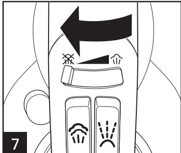
To turn iron off, set Adjustable Steam Control to (Dry Iron).
