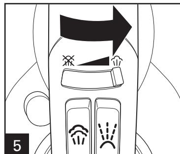
Set Adjustable Steam Control to the desired steam level.
