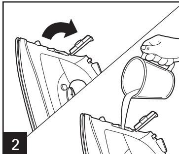
**Water:** Use ordinary tap water. If using extremely hard water, alternate between tap water and distilled water. DO NOT add starch or fragrance to the water tank.
