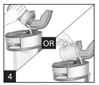
Water reservoir has two water levels: one for 8 oz. (250 ml) (minimum) and one for 14 oz. (410 ml) (MAX line) of water.
