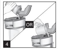
Water reservoir has two water levels: one for 8 oz. (250 ml) (minimum) and one for 14 oz. (410 ml) (MAX line) of water.
