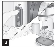
Replace accessories. Run two to three cycles of cold tap water. The unit is now cleaned and ready to make coffee.
