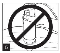
**NOTE:** Do not immerse the motor unit past the top metal portion of each attachment.
