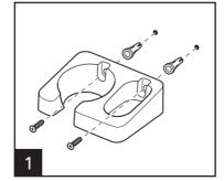
Attach wall mount to wall using the included anchors and screws.
