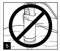
**NOTE**: Do not immerse the motor unit past the top metal portion of each attachment.
