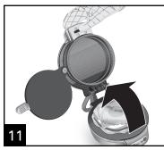
Using an oven mitt, lift ring assembly and cover by holding bottom handle to open. Some sandwiches are easier to remove if rings are lifted individually.
