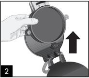
To remove ring assembly for cleaning, hold bottom handle to open, and then lift straight up.
