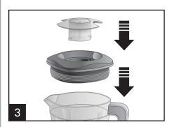
Place lid and emulsion cup on jar. Insert the cup into the lid and secure by turning clockwise. Remove the emulsion cup to use the tamper or to add ingredients.
