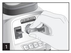
Rotate the VARIABLE SPEED DIAL to 1.
