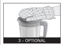
AWARNING Burn Hazard: Do not fill blender jar with hot liquid beyond the 1400ml level. With the protection of an oven mitt or thick towel, place one hand on top of lid. Keep exposed skin away from lid. Start blending at lowest speed.
