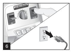
At the end of the blending cycle, rotate the VARIABLE SPEED DIAL back to the 1 position and press the START/STOP (♦/๑) switch to stop blending. Turn off the blender with the RESET/OFF (I/O) switch on the right side of the base. Unplug blender after blending.
