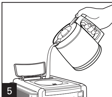
5 Lift water reservoir fill lid and add water.
