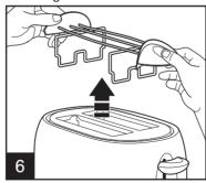
Remove rack after toaster is cooled completely.
