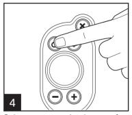
Select programming button after the bread lifter has been pushed down (if desired).
