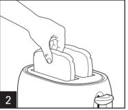
Plug into socket. Push bread lifter down to energize toaster and illuminate display. Press – or + to adjust toast shade.
