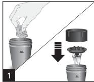
Add ingredients (no more than 1/2 cup [237 ml] or to the MAX fill line)to grinding cup. Carefully place cutting assembly and collar onto cup.
