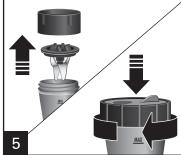
Turn bottom up, remove collar and cutting blade assembly from cup. Hand-tighten shaker/storage lid onto cup.
