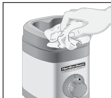
3. Wipe blender base, control panel, and cord with a damp cloth or sponge. To remove stubborn spots, use a mild, nonabrasive cleanser.
