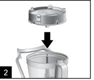
To insert the dicing assembly, lower the dicing disc onto the motor shaft, making sure the removable grid is next to the handle. Then lower the cutting disc onto the motor shaft until it sits flush to the dicing disc. TIP: When using the feed chute to dice, slice, or shred, make sure no other blades are in the bottom of the work bowl.
