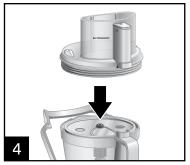
Place work bowl on base with handle facing forward. Adjust disc to desired thickness by turning the adjustment post. There are 14 adjustment positions, ranging from 1/32" to 1/4" (0.8 to 6 mm) thickness.
