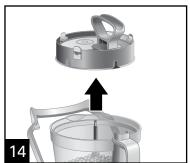
Remove dicing disc from motor shaft by grabbing metal clips.
