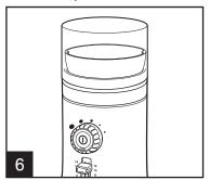
Place grinding cover onto grinder. Make sure the arrow on cover is aligned with the unlock symbol on back of grinder. Turn lid clockwise to locked position. Grinding cover will "click" when locked into position.
