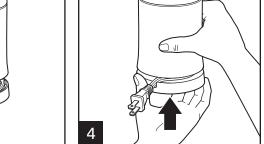
Hold coffee grinder in one hand and pull down on the base with your other hand. Wrap cord around hidden area of base. Place cord in cutout of base, leaving the plug outside the base. Push base up to store cord.
