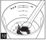
Use a small soft-bristled brush to remove grounds at the bottom of the grinding chamber. Blade is sharp, don't touch it by finger.
