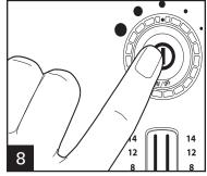
Move switch up or down to select the amount of cups you will be brewing. Turn grind setting dial clockwise to select COARSE, MEDIUM, or FINE grind. Refer to charts on page 5 for grinding and cup selection. Press the ON/OFF (①) button to start grinding. Grinder will turn off automatically at the end of selected grind.
