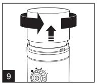
Lift cover straight up to remove. If locked in place, turn counterclockwise to unlock; then lift straight up.
