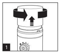
Remove grinding cover, if locked in place, by turning counterclockwise to unlock position; then lift straight up.
