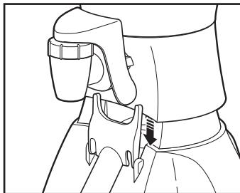
**NOTE:** The cutting assembly must slide between the base and dispensing lever to allow the lever to operate the dispenser.
