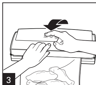
3 Close and hold lid; then press Vacuum & Seal button. Continue holding lid closed during entire vacuum and sealing process.
