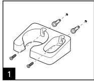
Attach wall mount to wall using the included anchors and screws.
