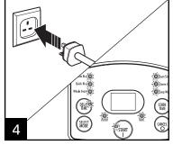
Plug into wall outlet; all lights will flash on control panel. If program is not selected, OR after pressing **CANCEL (O)**, the rice cooker control panel will flash for 15 seconds and the rice cooker will turn off.
