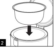
Pour desired amount of water in cooking pot. Carefully place cooking pot straight down on base. Make sure cooking pot is securely seated by rotating the pot left and right.
