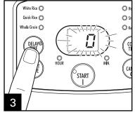
Press **DELAY TIME**. The display will flash "0." Continue to press **DELAY TIME** to set delay time from 1 to 15 hours. Press **START (I)** to begin delay start countdown or rice cooker will automatically start after 5 seconds.
