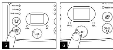
Press **SELECT MODE** to select White Rice, Quick Rice, or Whole Grain function. Light will glow for function selected. Press **START (I)** to start cooking OR unit will start automatically in 5 seconds.
