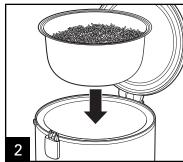
Carefully place cooking pot straight down on base. Make sure cooking pot is securely seated by rotating the pot left and right. **NOTE**: Make sure bottom of cooking pot is not bent or warped, or it will not conduct heat correctly.
