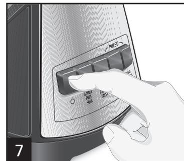
Push the desired speed button. When using the PULSO (Pulse) button, the blender will only run when the button is held down.
