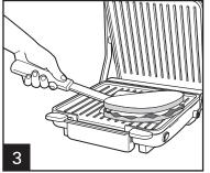
When preheated, raise cover, Place food to be cooked onto cooking grids and lower cover to desired height. Lock cover at desired height by turning locking knob, if desired.
