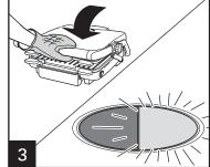
Preheat panini press for 6 minutes with cover closed. Once the grill has reached the proper temperature, the green light will come on.
