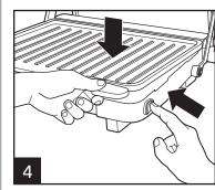
Replace cooking grids and ensure they are locked into place. ALWAYS replace LOWER cooking grid first. Repeat with UPPER arid.
