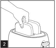
Plug into socket. Push bread lifter down to energize toaster and
