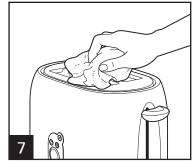
To remove food that becomes lodged in food slots, unplug from socket and allow toaster to cool. Turn toaster upside down and shake. Do not use fork or other utensil that could damage heating element or result in risk of fire or electrical shock.
