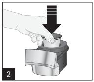
Plug in unit. Remove the coffee drawer. Add single-serve pack to single-serve pack holder (compatible with K-Cup pack such as UCC or Starbucks\*). Press down until flush with top surface.
