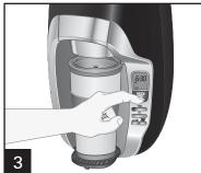
Press button, After 60–90 seconds, press button to stop the brew cycle. Allow the vinegar solution to steep for 30 minutes to loosen built-up minerals. Press button to finish the brew cycle. Empty remaining vinegar solution from reservoir, add fresh, cold water, and brew several cycles to empty the water reservoir, which will clean the system.
