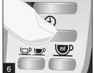
To adjust minutes faster, press and hold (4) button. Release button and wait 3 seconds for the clock to stop flashing and the time will be set.
