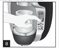
Press to select cup size and press or to select regular or bold strength. **NOTE**: Bold setting should be used for single-serve packs and ground coffee for a more robust flavor. Press (ON/OFF) to brew your coffee. Button will illuminate and will turn off when brew cycle is complete. Rinse coffee drawer. Then put drawer back into coffee maker.
