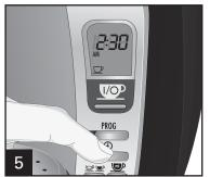
Minutes will flash for only 3 seconds and then stop flashing if the clock button is not pressed or held within that time. Press (4) button to adjust by 1-minute increments.
