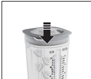
5. Push lid fully down into jar and ensure filler cap is secure by turning clockwise.
