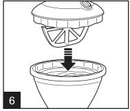
Ensure lid with motor housing is securely placed on freezer bowl. Plug into socket. Press switch to ON (I).
