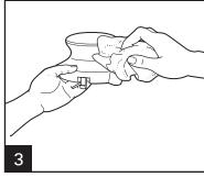
Wipe motor housing with a damp cloth. Do not immerse in water or other liquid.
