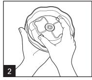
Squeeze locking tabs and remove motor housing from lid.
